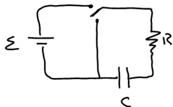
Switch up — charging RC circuit
