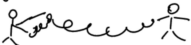
Observe the transverse wave travel along the Slinky. (might want to make this displacement in the horizontal direction if the Slinky is touching the floor.)
