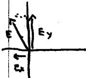
$$E_x = -\frac{\partial V}{\partial x} = -\left. \frac{dV}{dx} \right|_{y=\text{const}} = -2 \text{ N/Coul}$$
