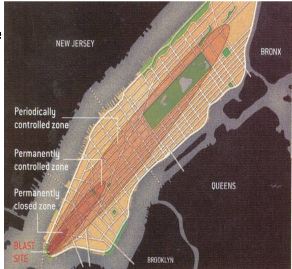
Figure 6. A simulated effect of detonation of dirty bomb (3,500 curie of cesium-137 with ~50 lbs of explosive) at the lower tip of Manhattan Island (Scientific American, November 2002, page 76)
